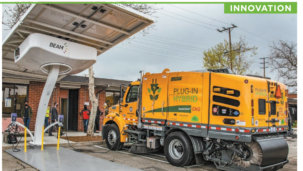
One of two plug-in hybrid street sweepers and the Beam solar-powered recharging station at the North Hollywood StreetsLA yard.
