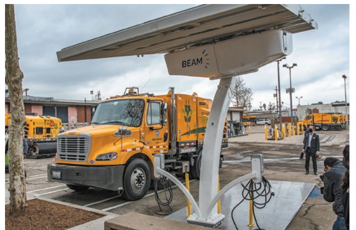
A hybrid plug-in street sweeper is ready to recharge at the Beam solar-powered charger.
