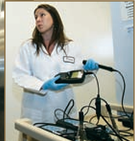
Water quality measurements (e.g. salinity, pH, dissolved oxygen) are performed using probes throughout the duration of the toxicity tests.
