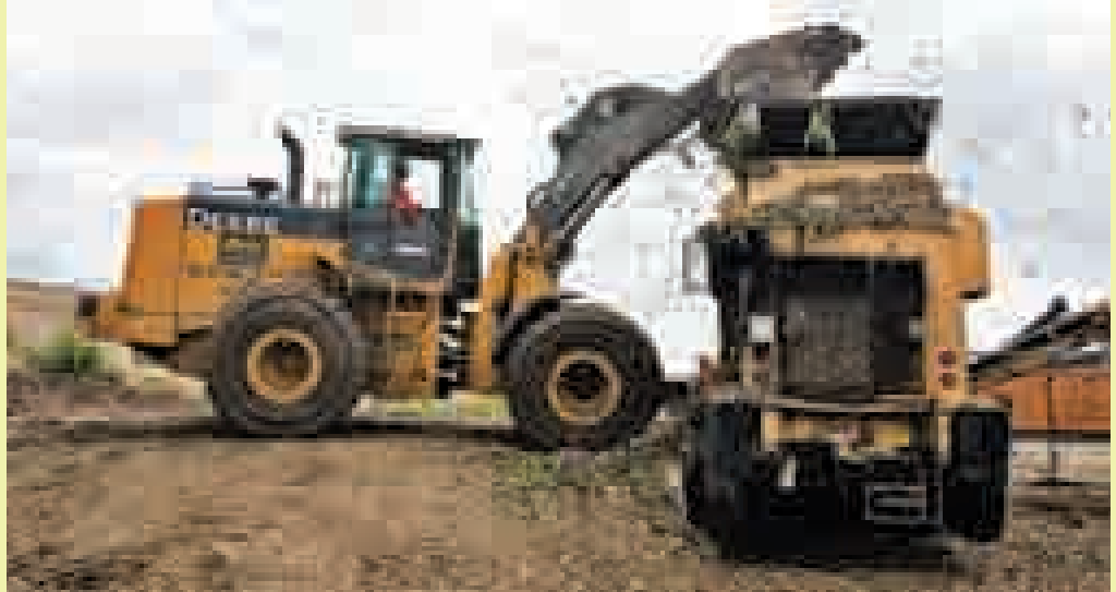
Anceo Francisco, Equipment Operator, dumps raw mulch into the trommel screen machine.
