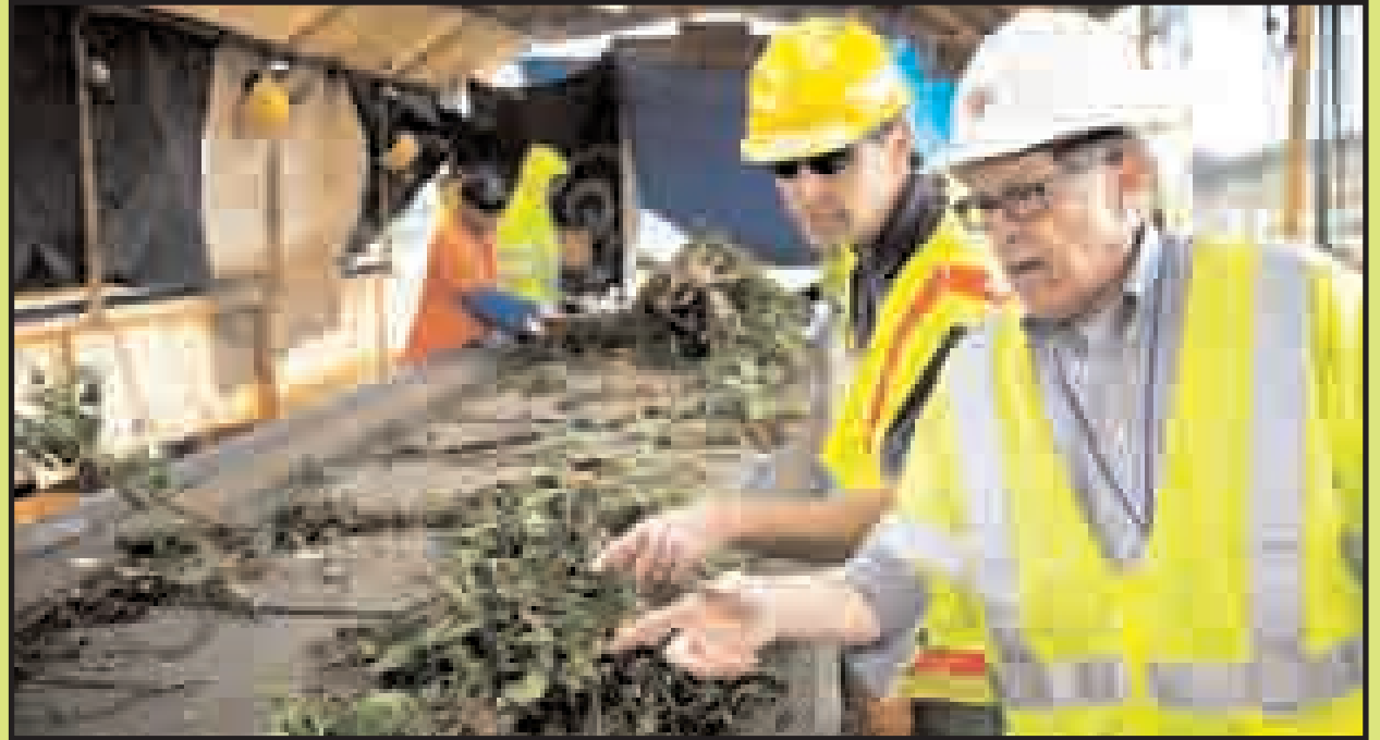
Paul Blount, Operations Manager (right), describes how solid contaminants (bottles, paper, etc.) are picked by hand from the raw mulch, along a conveyor belt.
