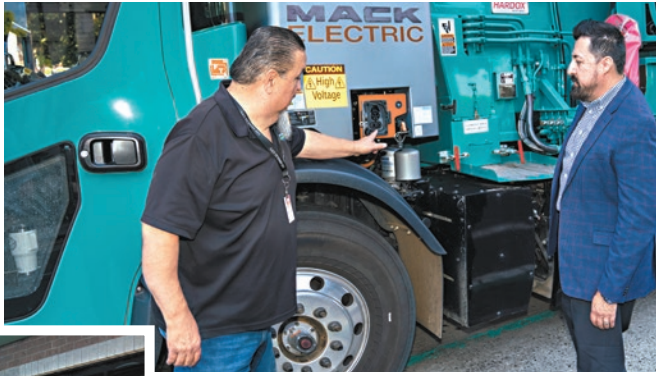
LEFT: The Mack automated side loader arrives for long-term testing by Sanitation. Automated side loaders do most of the heavy work of trash collection in the City of Los Angeles; employing a large fleet of fully electric automated side loaders is the goal in Sanitation's clean fleet plans. (This is the same vehicle on the cover of this month's issue.)
