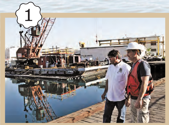
On the home dock, Anthony Di Tucci (left), Manager of Vessel Operations, explains to Club CEO John Hawkins what's going to happen – the derrick barge (in back) carrying the piles (just above the water) will be tugged by the City tug Yankee to the dock where they're needed. The derrick barge does not move under its own power.
