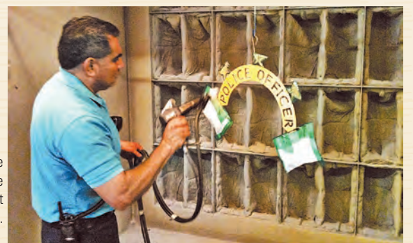
Powder coating the End of Duty badge that was installed at Foothill Division.
