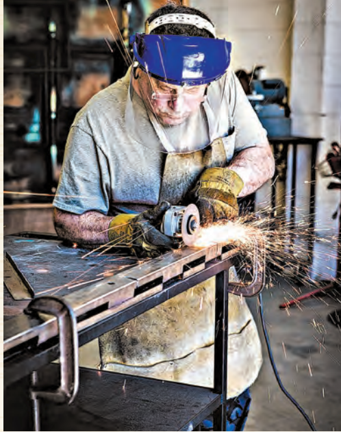
Rich Colton cuts tubular steel to create the frames for the City Seal.
