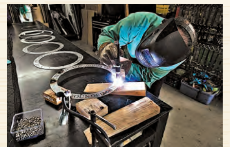
Tim Lampros welds bolts onto City Seals in production.
