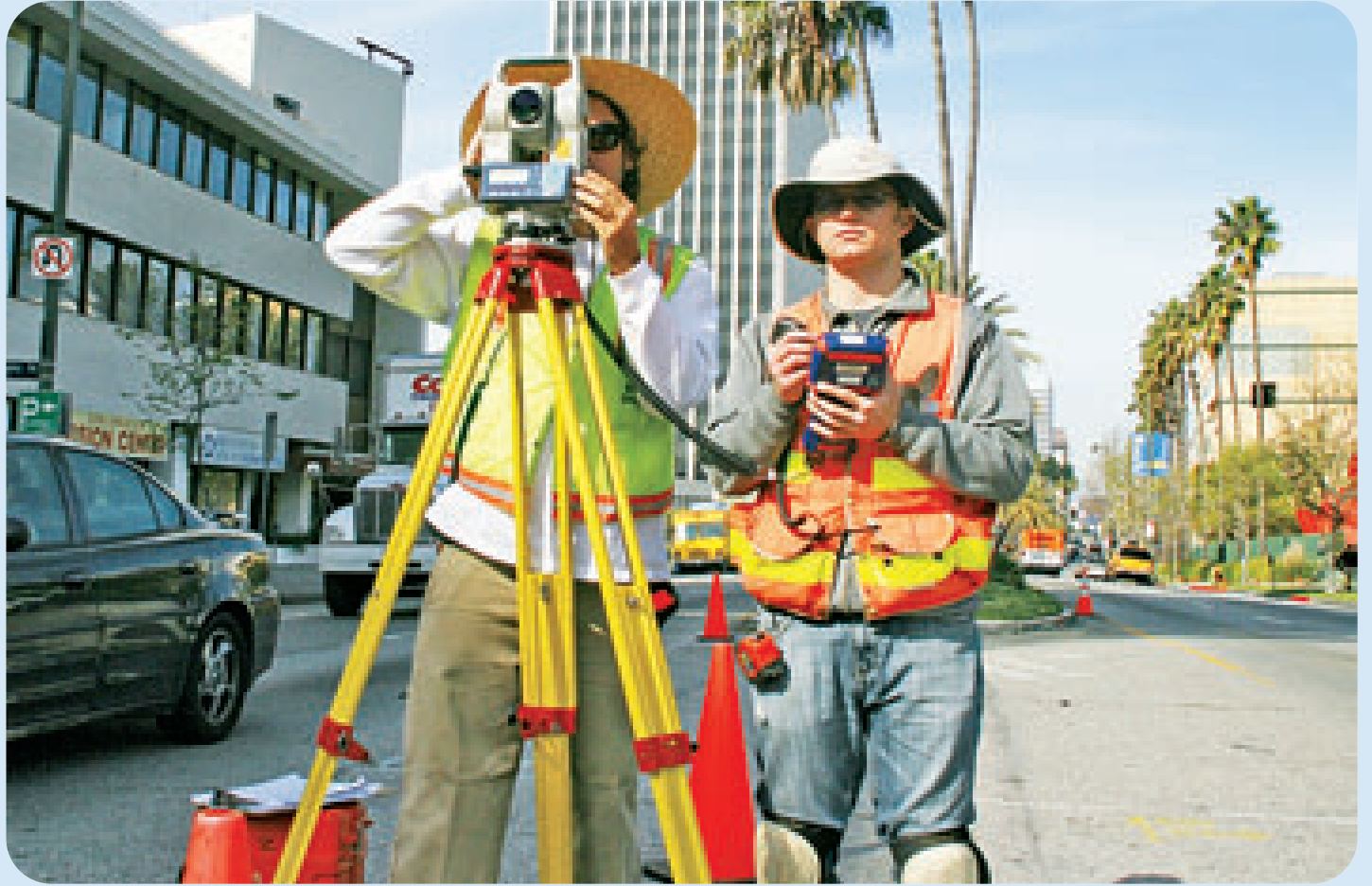
Survey crew at work collecting data that will be used for engineering the new Wilshire Bus Only Lane project.
