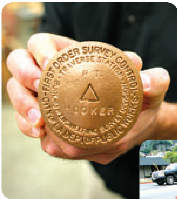
ABOVE: Club CEO John Hawkins holds a monument stored in a Survey Division warehouse that's ready to be installed on a City street. The City has more than 96,000 monuments similar to this one installed in the City.
