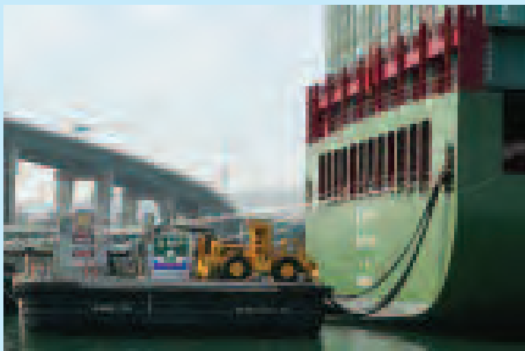
The Port's AMP project allows cargo ships in dock to connect to electricity from the dock, rather than running their own diesel engines. This creates far less pollution for the Harbor air.
